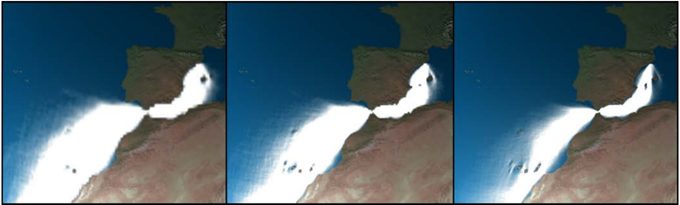
Figure 1: Render to a texture results. Texture resolutions and frame rates, from left to right: 1024 res, ~50 fps; 2048 res, ~43fps; 4096 res, ~35 fps.
