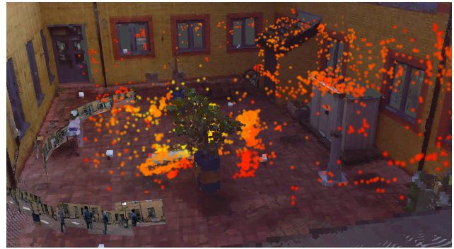
Figure 5: Camera coverage point cloud superimposed on the LIDAR set data. Bright yellow points are seen by more cameras, dark red points are seen by fewer.
