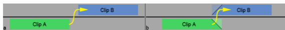
Figure 4. Figure shows how blending can be made between two clips. Left: interpolating from last frame of Clip A to first frame of Clip B; or Right: cross fading from Clip A to Clip B.
